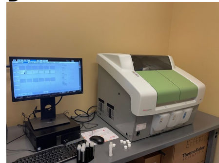
Figure 1 A: Curio micro malter and kiln to achieve experimental levels of germination and modification for malt quality analysis. B: WSU elite lines from the germination tanks to be kilned. C: Congress wart extraction. D: Robotic ThermoScientific Gallery analyzer for high throughput analysis of Beta glucan, Alpha Amylase, Extract and Diastatic power.
