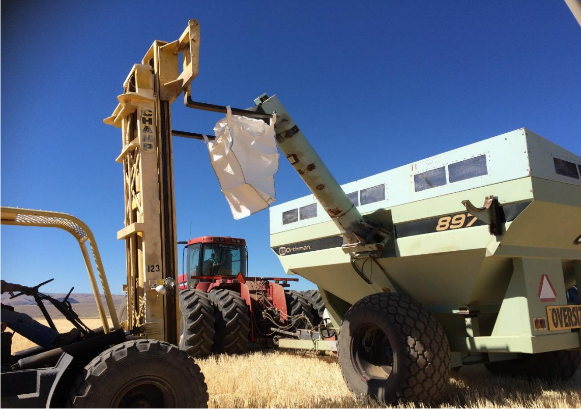
Figure 4 Transferring a 500 lb subsample from the weigh wagon into a tote sack.
